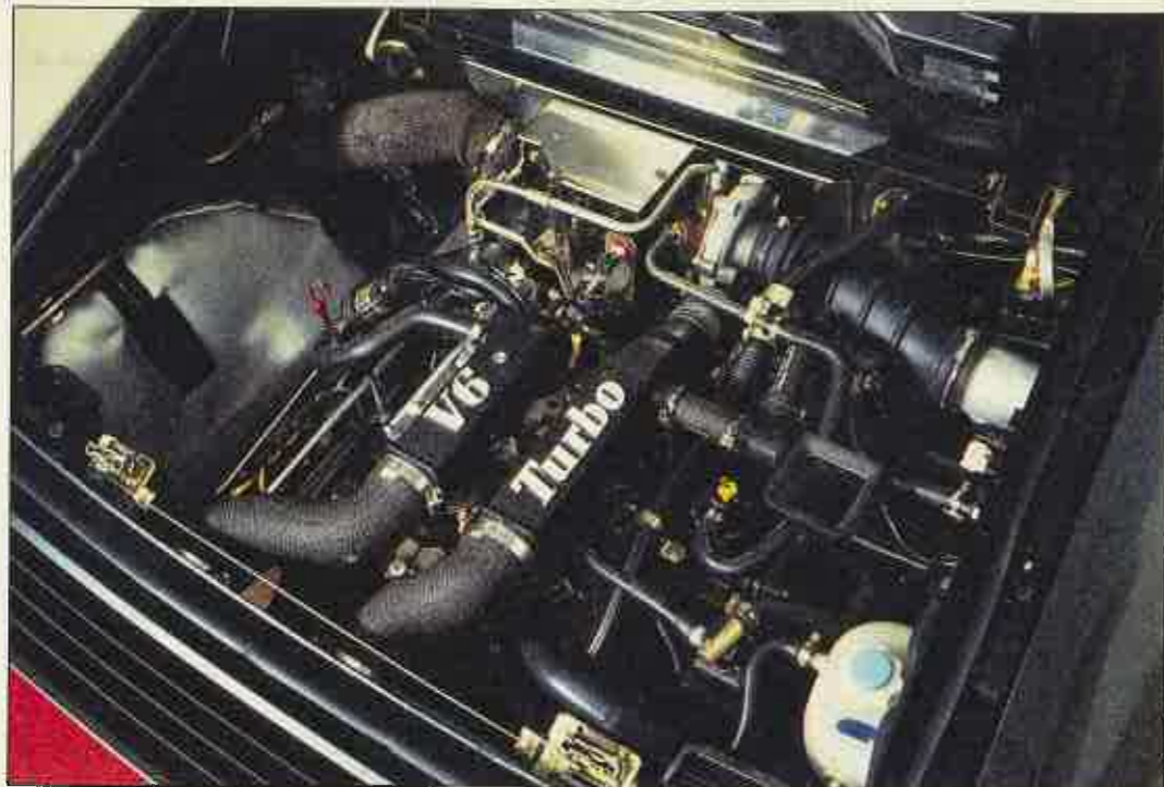
The turbocharged, intercooled 2.4-litre V6 (left) traces its ancestry back to Renault's F1 engine and is refined and flexible. The cockpit (left, centre) is well laid out with the exception of the pedals, while the front seats (bottom, left) provide comfort and excellent support. The nose compartment (below) is shared by the fuel tank and a tiny 'boot,' while the aggressive frontal treatment (bottom) leaves no doubt as to the GTA's considerable abilities.
